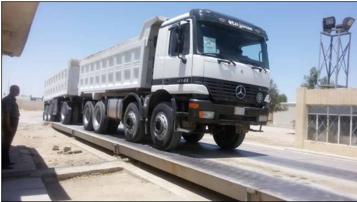
Fig. 1: Axle load survey of (11.22+2.22) trucks in Kerbala silo permanent weighing station.
