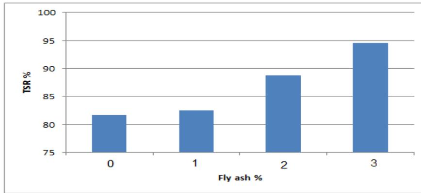
**Figure 5. Effect of fly ash content on tensile strength ratio**
