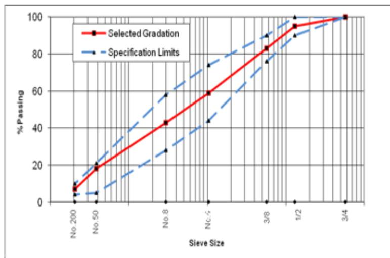
Figure 1. Aggregate Gradation.
