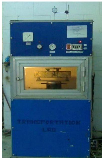
**Plate 3. Specimen Setup in the Testing Chamber**
