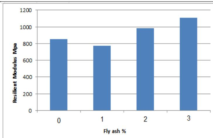
**Figure 6. Effect of fly ash content on resilient modulus**
