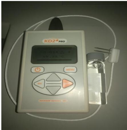
**Figure 3** KD2PRO measuring device for thermal conductivity of nanofluid produced by DECAGON DEVICE INT.
