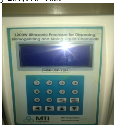
Figure 2 1200W Ultrasonic processor for homogenizing nanofluid produced by MTI CORPORATION.
