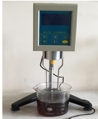
Figure 4 NDJ-5S Viscometer measuring device for dynamic viscosity of nanofluid.
