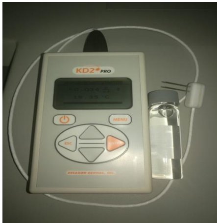
Figure 3 KD2PRO measuring device for thermal conductivity of nanofluid produced by DECAGON DEVICE INT.
