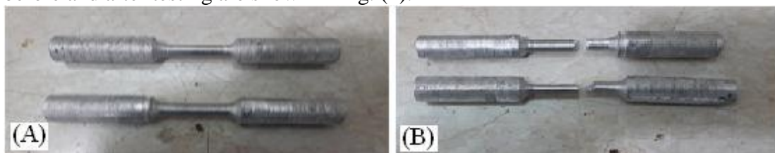
Fig.(4) Tensile specimens: (A) Before testing (B) After testing
