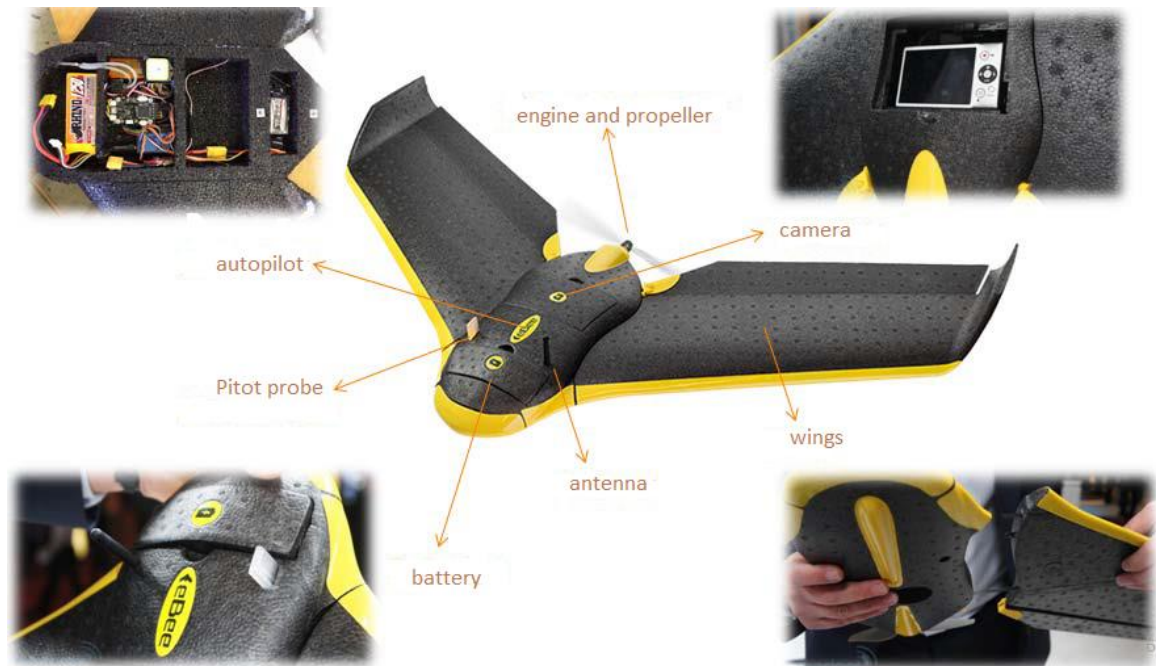
Figure 5: Elements of Unmanned Aircraft Ebee (sensefly, 2015)
