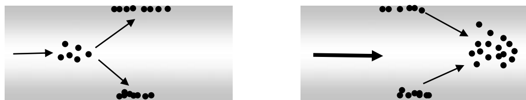
Figure 1: Processes leading to the occurrence of discolouration within water distribution systems (after Vreeburg and Boxall (2007)).
