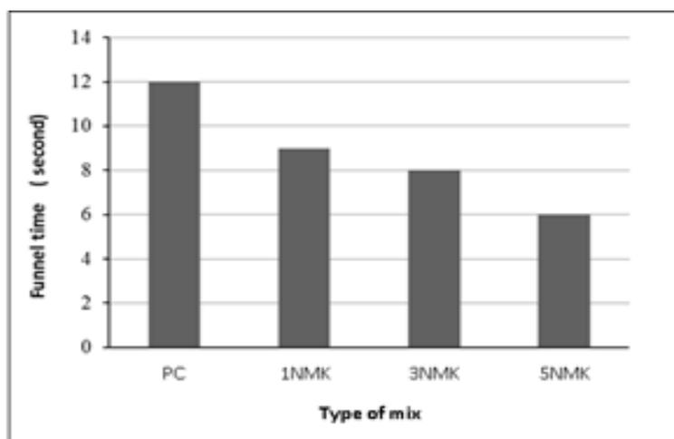
Figure (4): Funnel time of V-funnel for SCC at different percent of NMK
