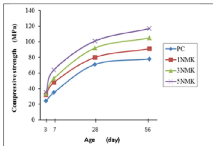
Figure (5): Relation between compressive strength and age for SCC at different percent of NMK
