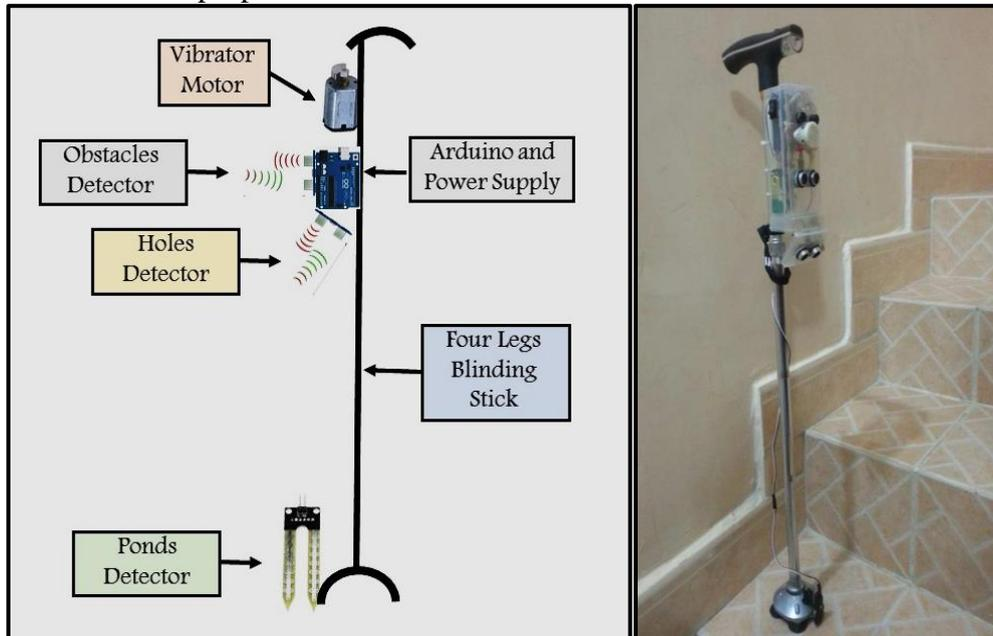
**Figure 1 Proposed Smart Blinding Stick System.**
