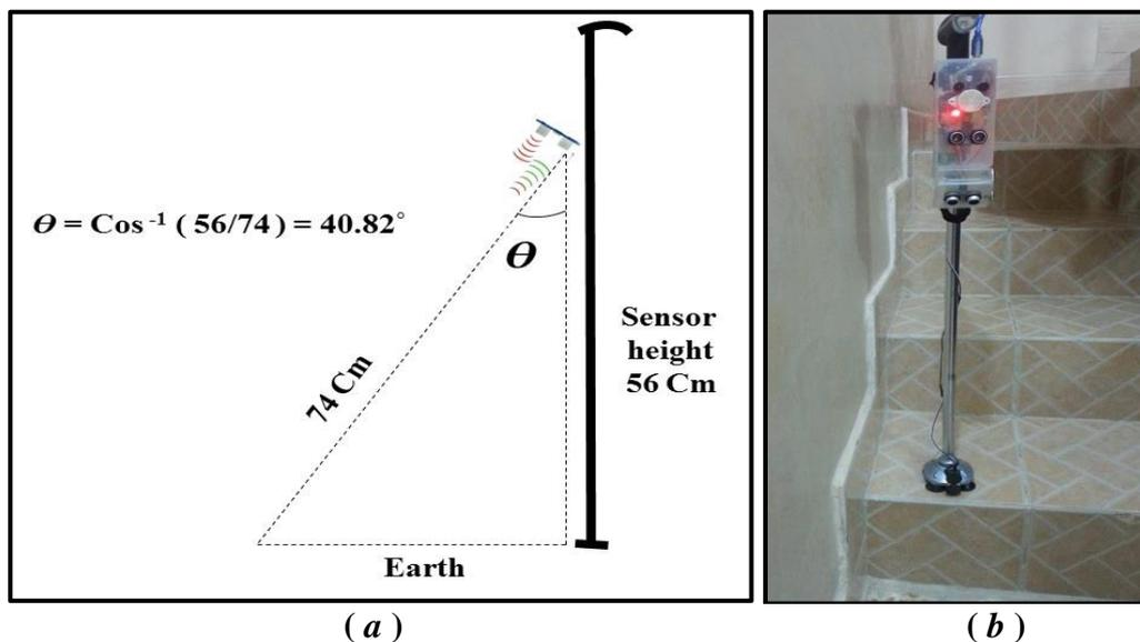
**Figure 6 Holes Detection Process and angle measurement.**
