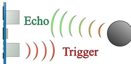
**Figure 4 Ultrasonic sensor work**
